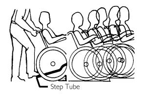
FIGURE 2.3 Method I - Wheelchair With Step Tubes
